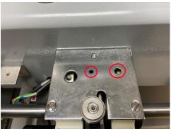
3. Remove the cover in-between Head #1 and Head #2 before continuing on with step #4
