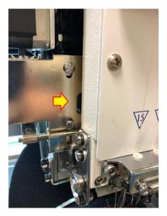
When oiling inside this hole, you are to hit the two points highlighted below:
