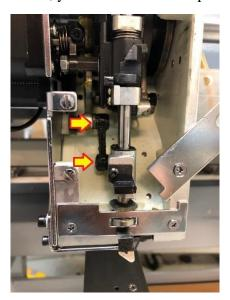
5. Needle Bars (springs behind take up levers)-1 drop on each needle bar spring weekly
