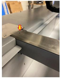
8. Thread Holding Device-Using the Alba-5 Lubricating Spray, spray the thread holding device from underneath it (roughly two or three sprays to cover all 15 needles) once per month
